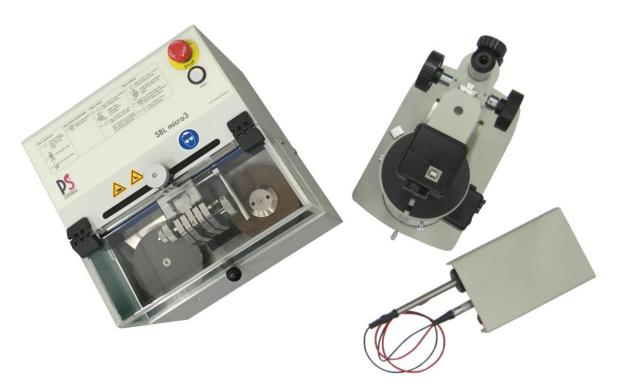
**SBL micro3** – a compact and user friendly portable micrograph lab, all-in-one combined with AUTOMATIC cutting + polishing module, reduce processing time to cater for the ever increasing quality demand. Stand alone Etching module and full size Imaging module that gives high quality imaging results for a clearer, more accurate cross-section analysis through X5 vision – Evaluation & Documentation module.
